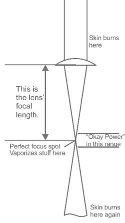
The classical way to test focus is to set up some material purposely slanted so the laser hits it at different distances from the lens. If you do this right, you can lase multiple lines and pick the thinnest line. That's very near the true focus length. Then you set up your bed so new sheets of material are close to this perfect distance.
